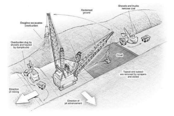
The following diagram illustrates a typical dragline surface mining operation:
