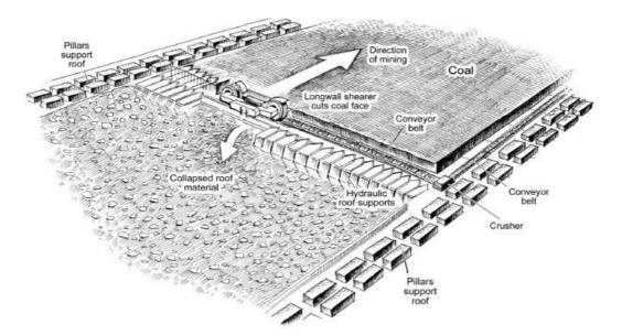
controlled fashion. The following diagram illustrates a typical underground mining operation using longwall mining techniques:
