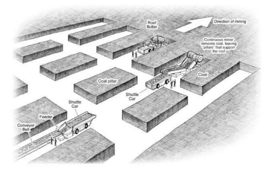
The following diagram illustrates our typical underground mining operation using room-and-pillar mining techniques:
