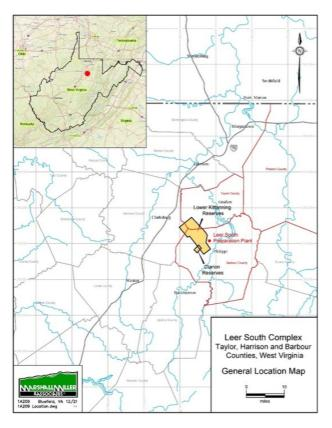
Leer South consists of the newly commenced longwall Leer South operation in the Lower Kittanning seam, existing Sentinel underground mine in the Clarion seam, a preparation plant and a loadout facility located on approximately 26,000 acres in Barbour County, West Virginia.
