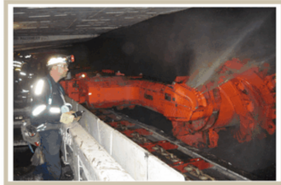
(shearer at the longwall face)
